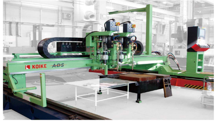
CNC Piercing hole drill specialized machine specialized in piercing holes where cutting is necessary.
